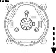
MOUNT ASPC-2 WITH THE SAMPLE LINE CONNECTIONS IN THE "DOWN" THROUGH AT LEAST TWO OF THE FOUR MOUNTING FFFT HOLES.
